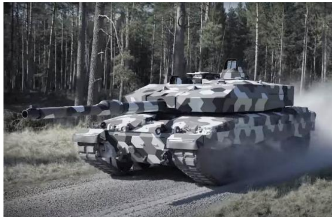
The new Rheinmetall Main Battle Tank MBT with its new armor and 130mm gun (Picture source: screenshot of Rheinmetall's video broadcasted on July 31, 2020)
