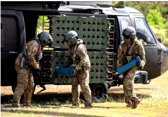
Soldiers from the 25th Combat Aviation Brigade train with the Volcano system on a UH-60 Blackhawk at Makua Range, Hawaii, June 23, 2020. (Net. Sarah D. Sauersteiner/Army)
